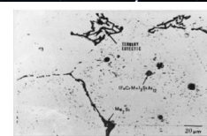
Micrograph of cast 6061 showing Mg 2 Si, complex intermetallic, and ternary eutectic phase. From Skollanos et al., Materials Science and Engineering A231 (1997) 17-24
