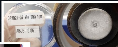
1. Aluminum propellant rod in pulsed plasma thruster test bed.
