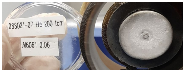
Figure 3. Aluminum propellant rod in a vacuum arc thruster test bed.
