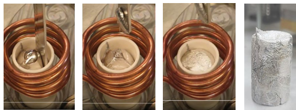
Figure 1. Steps of the rod forming process.
